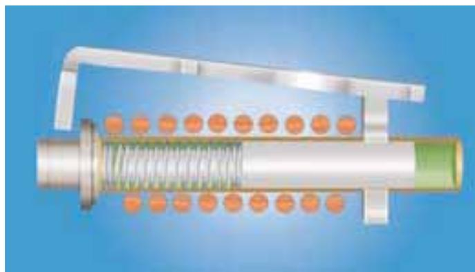
**Figure 3: Overload Current (Time Delay)**
